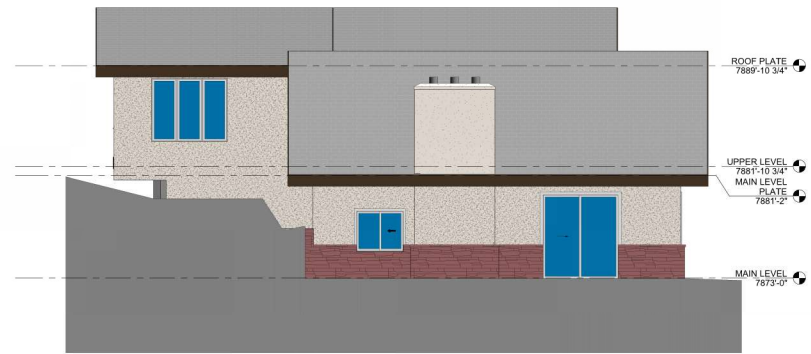
3 WEST ELEVATION - EXISTING 1/4" = 1'-0"
